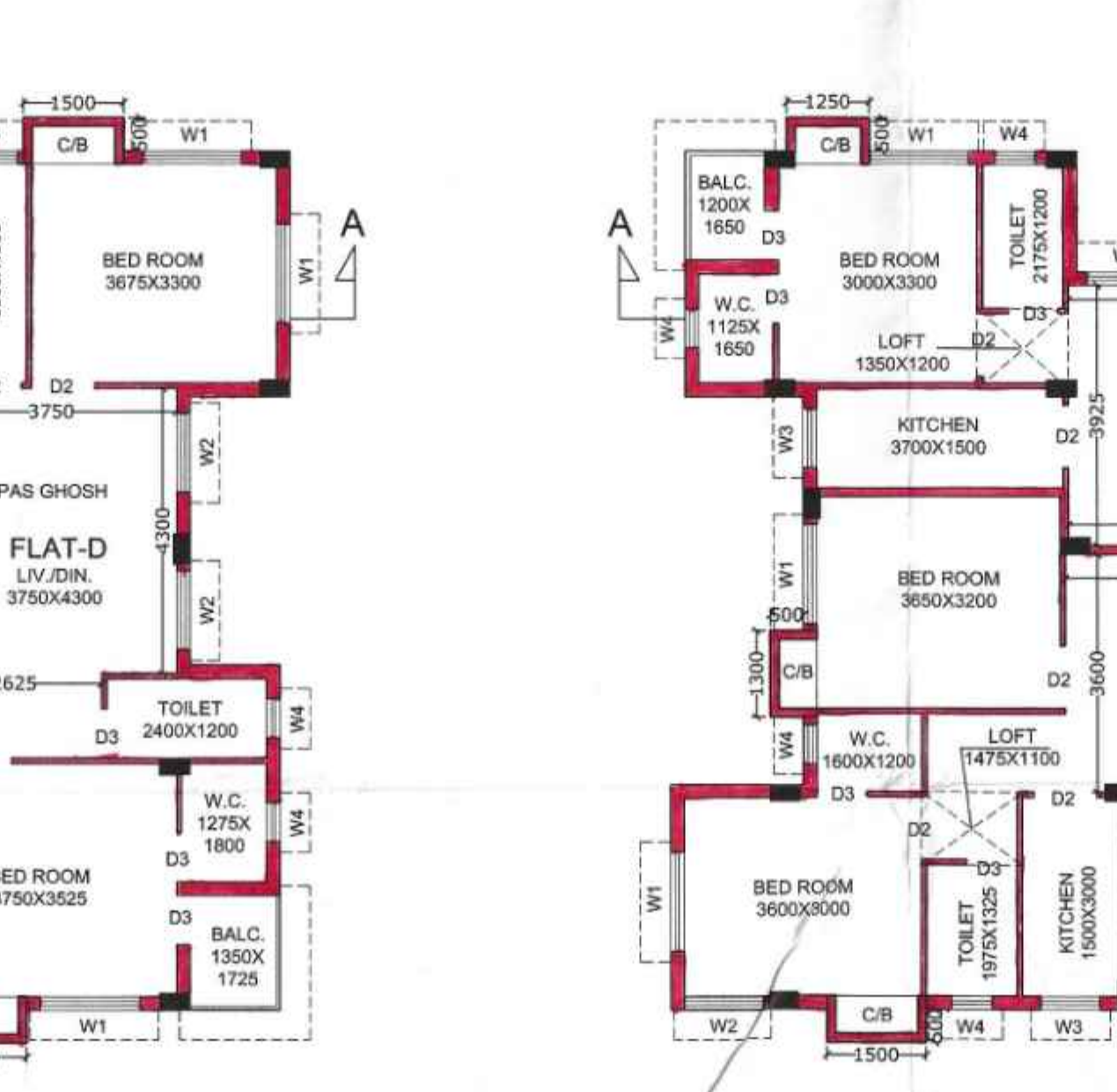
PROPOSED SECOND FLOOR PLAN (OWNER'S ALLOCATION) SCALE: 1:100
